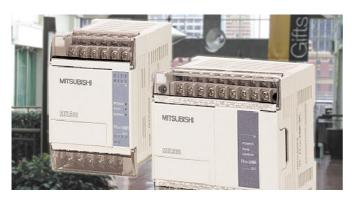
Designed and supplied by Keltron the KCL S90C addressable control system works alongside the mandatory fire detection system. At the heart of the Keltron control system is a Mitsubishi Electric FXON programmable logic controller (PLC). This controls via the KCL S90C communications interface as many as 100 distributed field units which monitor or control sensors, fire or smoke dampers and fans via a two-wire fieldbus network at locations up to 2km from the central controller.
