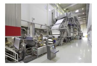
A condition monitoring system installed on a paper coating machine has enabled the Mitsubishi HiTec Paper Europe plant in Bielefeld, Germany to switch from time-based to condition-based monitoring, helping to avoid unnecessary machine shutdowns. Enabling the new system is a Mitsubishi Electric L-series PLC that operates as a bidirectional gateway between the controller and sensors.
