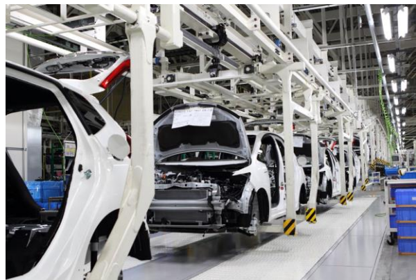
Picture 2: By introducing cutting-edge production technology, the Honda Yorii Plant has achieved a tact time of less than 50 seconds for the production of the FIT.
